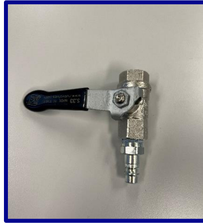
Fig.3: Images showing the 3/8 th quick connector to be mounted on the air hose.
