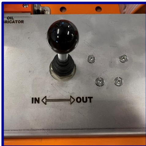
Fig.7: Images showing turning ON the main air inlet valve.
