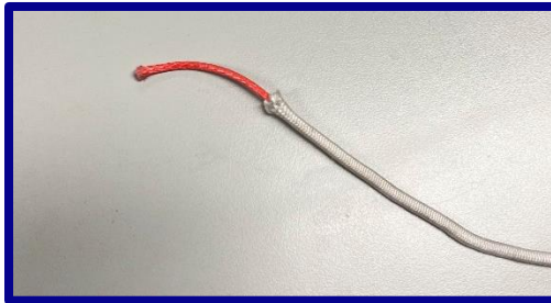
Fig.13: Colored core of rope. Cut or replace if visible.
