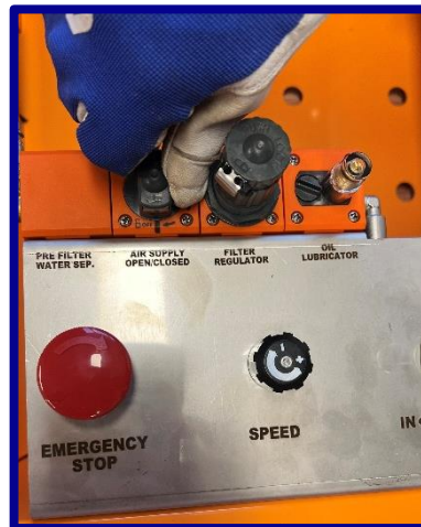
Fig.7: Images showing turning ON the main air inlet valve.
