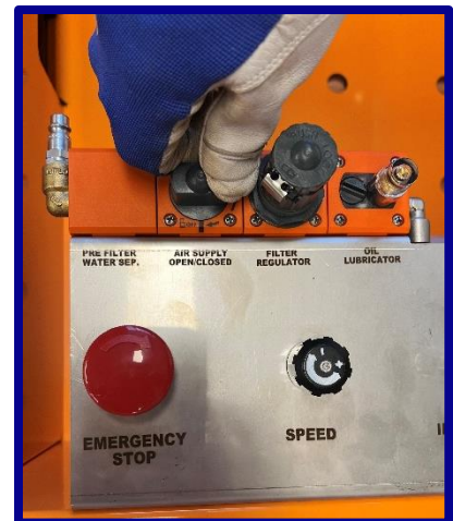
Fig.7: Images showing turning ON the main air inlet valve.
