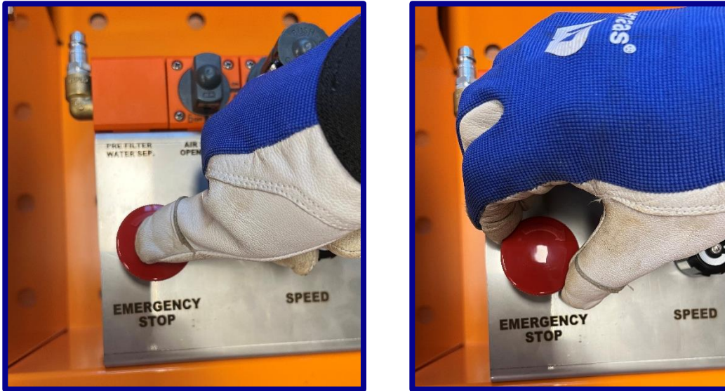
Fig.8: Images showing releasing of emergency stop switch.
