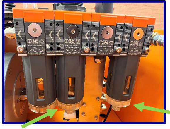
Fig.15: Drainage point below the filter unit pos 1 and filter/regulator unit pos 3.
