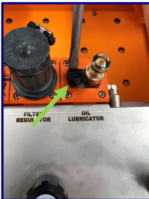
Fig.14: Opening the lubricator section and filling lubricant.
